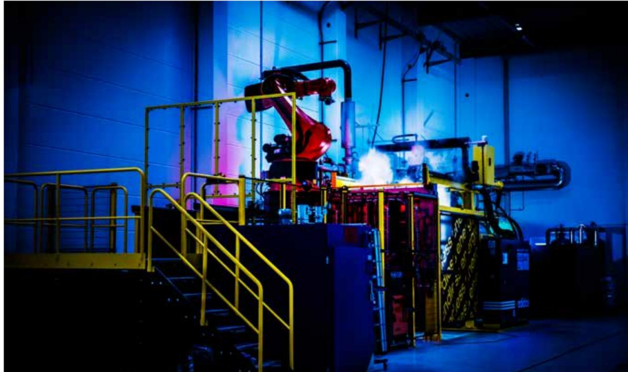
In just a few seconds, Speedfactory machines can heat and mold material into Adidas' running shoe soles, with a single worker required to wedge in pieces of plastic. Manual stitching and gluing are replaced with molding and bonding done by machines to roll out shoes in a day. Sneakers can also be customized by style and fit. More Speedfactories are planned for Atlanta, Paris, London, New York, Los Angeles, Tokyo and Shanghai in 2018.
