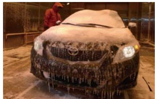
Evaluation under artificial cold-weather and snowing conditions
